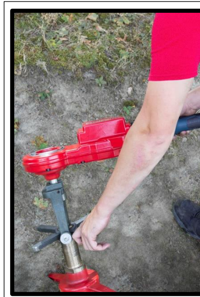
CPDWW turning a TM1100 Tapping Machine with a TMPDA Power Drive Adapter.
