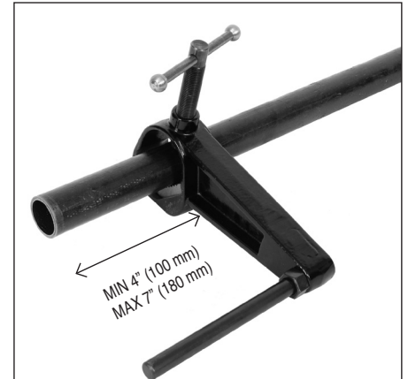
Fig. 5 Rod on black safety arm helps resist the threading torque to protect the operator.
