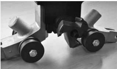
3. Tighten PVC Bevel Cutter onto Long Arbor
