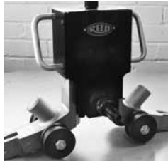
2. Tighten Long Arbor onto motor unit
