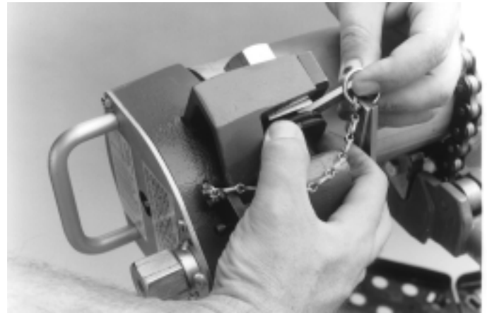
Fig. 3. Setting Gauge Depth
